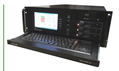
The Apollotek APK8780 series of Telemetry Groundstations and Data Recorders are designed to provide recording and replay of multiple serial PCM Streams as typically processed by internal Telemetry Receivers, Bit Synchronisers and Decommutators.
