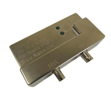
The Apollotek APK87611 is an IRIG-B Time Code Reader which is one of the Apollotek range of USB powered and interfaced products which are designed for PCM Flight Test Instrumentation system checkout and test and evaluation applications. The unit can optionally include an IRIG-B Time Code Generator (Specify APK87612 for this option). A GPS Receiver designed to extract time information from the received and decoded serial NMEA datastream is also available as an additional option.
